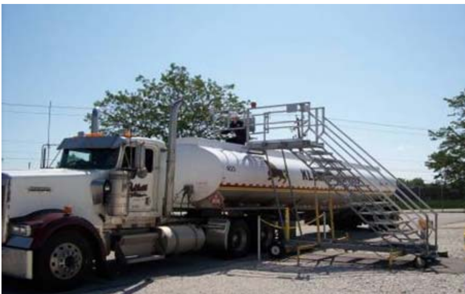
Stairway with a working platform is used to access the tanker hatch.
